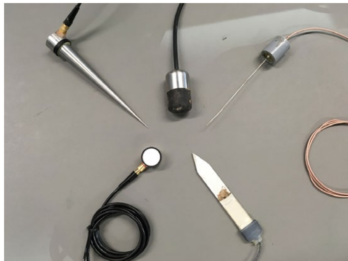
Fig. 2. Sounding Soil prestudy in summer 2016: Testing different acoustic sensors at the WSL, Birmensdorf/Switzerland.
