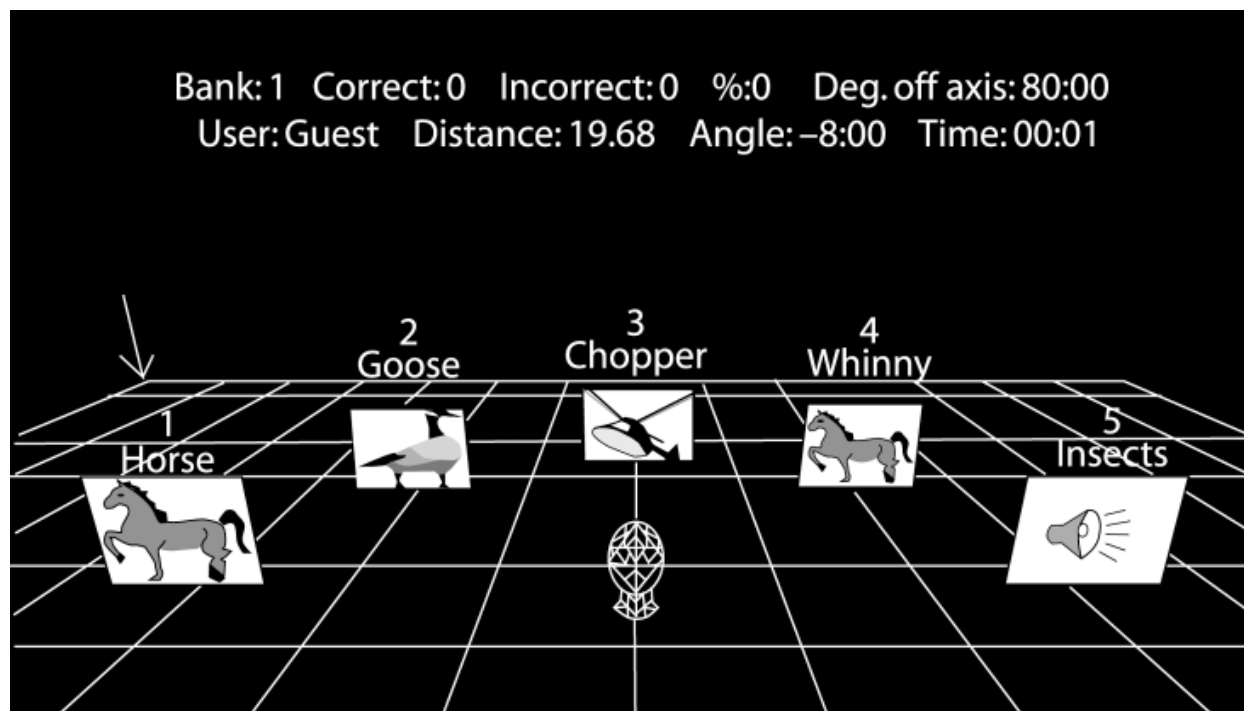
Figure 1: A screen shot from the virtual acoustic training software shows the orientation of the listener's head relative to other sounds presented in the environment. The 3-D environmental sounds can be moved, muted, or isolated with the software. As the student's head turns, the computer adjusts the perceived location of the environmental sounds in real-time.
