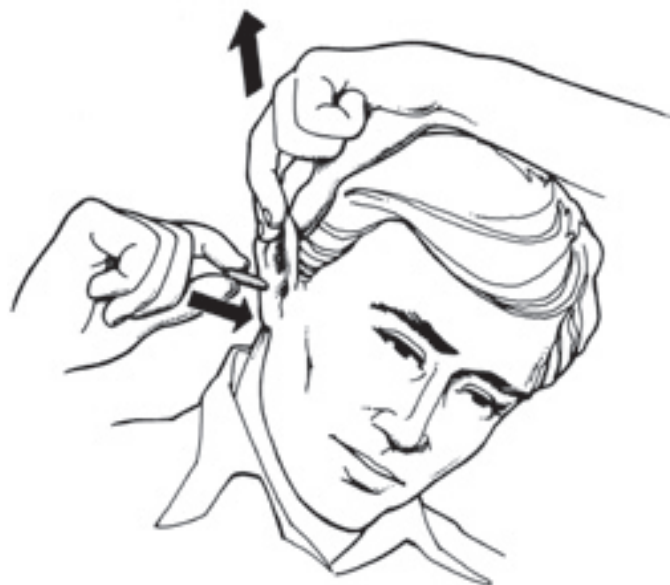
Figure 1—Illustration of the correct method of pulling the pinna (outer ear) by reaching over the head with the opposite hand to the ear being fitted.
